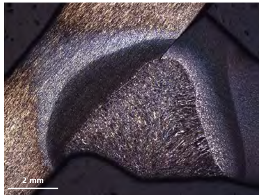
Laser weld, coaxial brightfield illumination, objective: 1.6x, magnification: 32x
